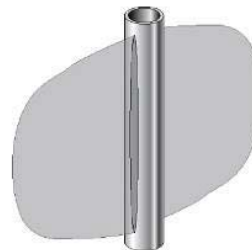
Figure 7—Least Principal Stress in the Horizontal Direction, Vertical Fracture
