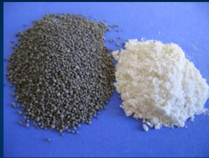
Traditional process DCP (left) with impurities and new process DCP (right)
